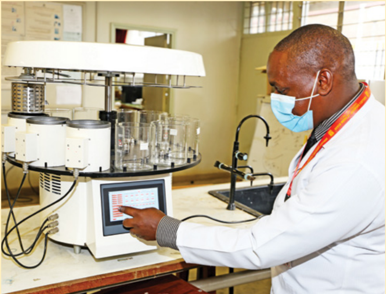
Medical Laboratory Sciences Lecturer Mr. Errols Sigei examines an automatic tissue processor used for practical lessons.
